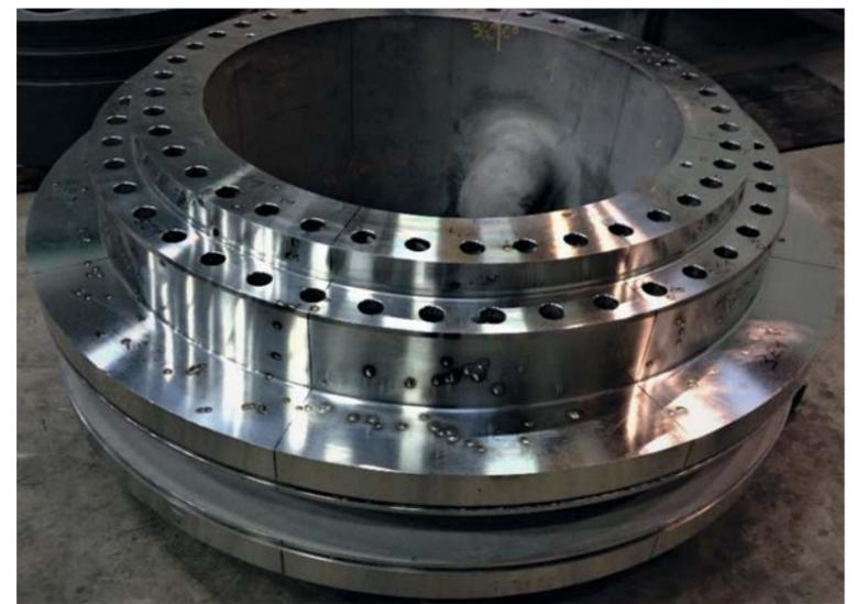
Figure 1 A casted duplex stainless steel inner housing of a swivel.
