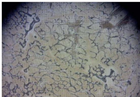
Figure 2 Duplex stainless steel after a poor heat-treatment.
