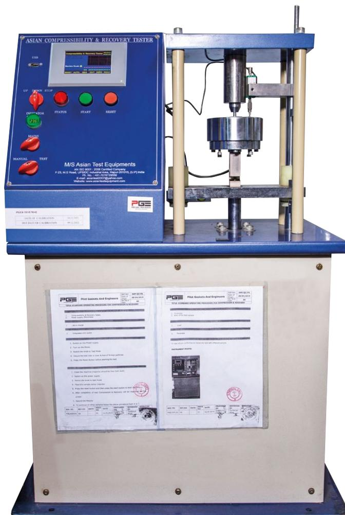
PGE has extensive in-house testing facilities, enabling the company to test materials under ASTM F36J, ASTM F146, ASTM F152, and DIN standards as well as to conduct extensive R&D
